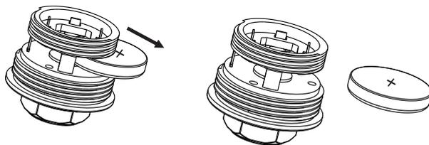
5. Replace the old battery with received, a new CR1632 battery cell, ensuring the positive+ is facing upwards.
