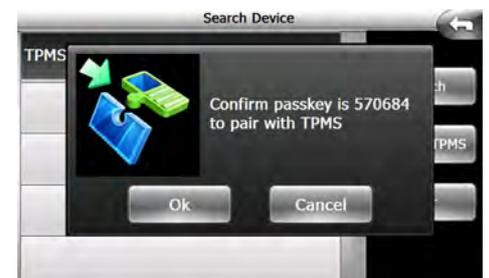
Pairing with Tyre Pilot STP1600/STP1800
