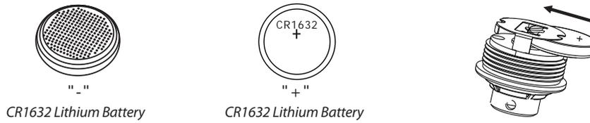
5. Check that the water-proof rubber seal is in the correct position. Screw the sensor cap back using the battery replacement tool to tighten.
