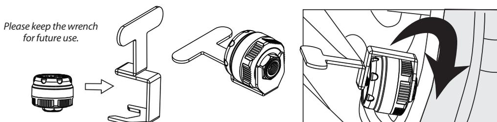
Do not over tighten the sensor cap to prevent possible damage.
