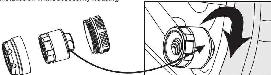
Do not over tighten the sensor cap to prevent possible damage.
