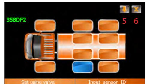
When the TPMS application is reopened you will see the tyre pressure readings (pressures shown here are for illustration purposes only)
