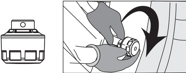
*Do not over tighten to prevent possible damage to the sensor.*
