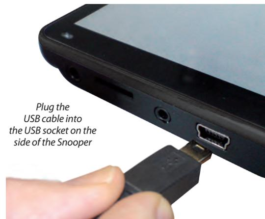
*Plug the USB cable into the USB socket on the side of the Snoopers*
