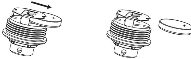
4. Replace the old battery with a new CR1632 battery cell, ensuring the positive+ is facing upwards.
