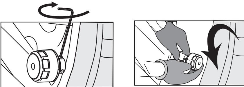
2. Use the battery replacement tool to unscrew the sensor cap.
