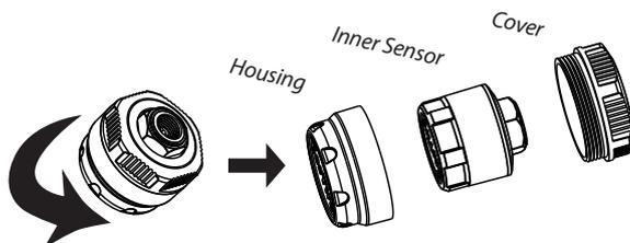
3. Use the wrench to open the sensor and gain access to the battery.
